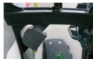
A cable feedthrough from the cab to the front and rear and a mounting rail on the right-hand door make it easy to install external implement control units.
