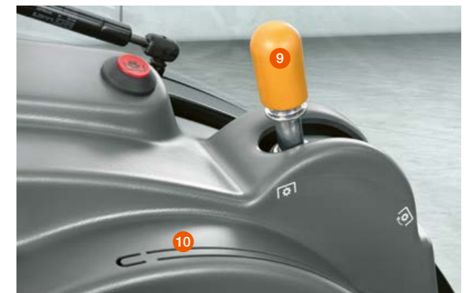
The PTO is engaged with hydraulic support as standard. Electronic PTO engagement is available as an option in machines with REVERSHIFT clutchless reverser and TWINSHIFT.
