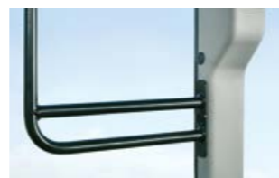
A cable feedthrough from the cab to the front and rear and a mounting rail on the right-hand door make it easy to install external implement control units.
