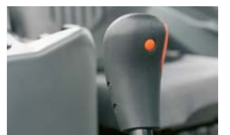
With REVERSHIFT and TWINSHIFT: the electronic clutch is operated by pressing a button on the gear lever.
