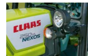
Folding side-marker lights on the NEXOS prevent damage to crops.
