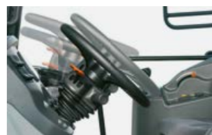
The steering column tilts and has telescopic height adjustment so it can be adapted to the driver's seating position.
