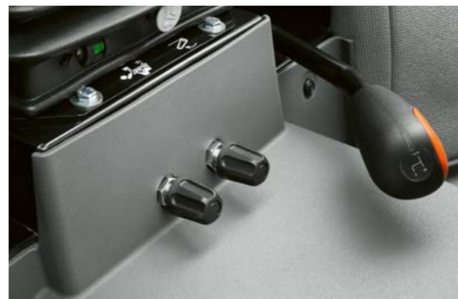
Even with the mechanical rear linkage, the lowering speed and draught control sensitivity can be finely adjusted under the driver's seat.
