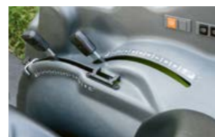
Choose between a mechanical and an electronic rear linkage control system. Both are ergonomically positioned to the right of the driver's seat.
