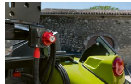
The battery isolating switch is easy to reach at the back of the cab.
