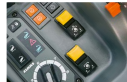
The front PTO is always engaged electronically. For the rear PTO, this function is available as an option.
