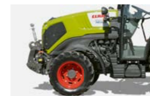
The folding front linkage reduces the overhang, allowing safe turning manoeuvres at the headland.
