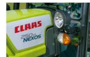
Folding side-marker lights on the NEXOS prevent damage to crops.
