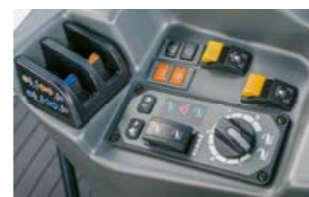
Choose between a mechanical and an electronic rear linkage control system. Both are ergonomically positioned to the right of the driver's seat.
