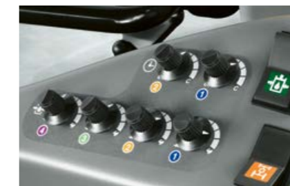
Time and volume control for the four electronic spool valves can be regulated at any time using the dials.
