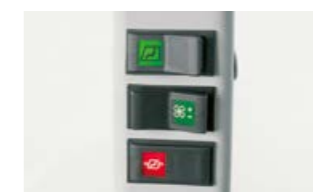
Status display for cab filter system and fan activation/control within easy reach on the B-pillar.
