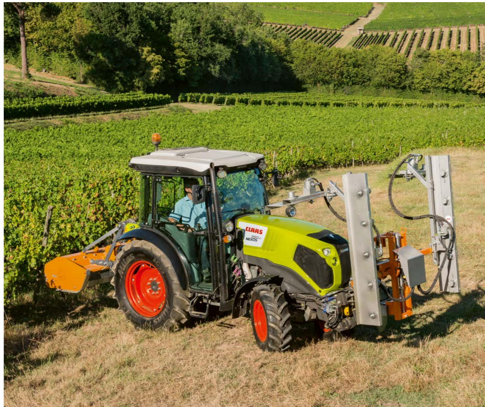
3-pump hydraulic circuit with a total flow rate of 114 l/min: 87 l/min for the spool valves and rear linkage and 27 l/min for the steering and transmission.
