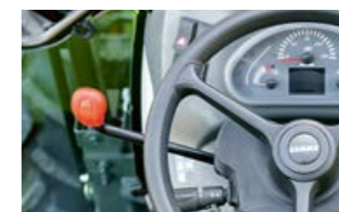
The reverser for mechanical reversing and the electronic REVERSHIFT are handily positioned to the left of the steering wheel.
