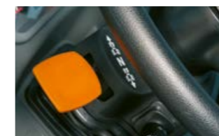
The reverser for mechanical reversing and the electronic REVERSHIFT are handily positioned to the left of the steering wheel.
