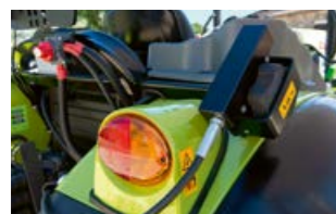
Convenient external controls with mechanical or electronic rear linkage.
