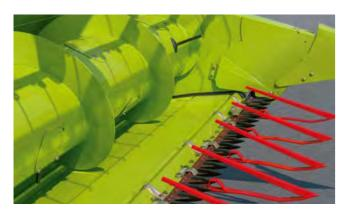
Cutterbar table retracted – grain (– 100 mm)
