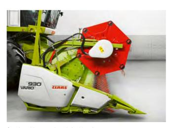
Cutterbar table retracted – grain (– 100 mm)
