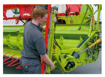
Rapeseed knives fitted by means of quick-release mounting system
