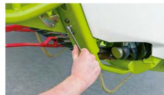
Easy adjustment of divider height using the panel key
