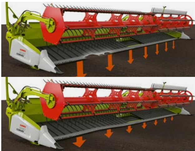
Ground pressure can be adjusted from the cab
