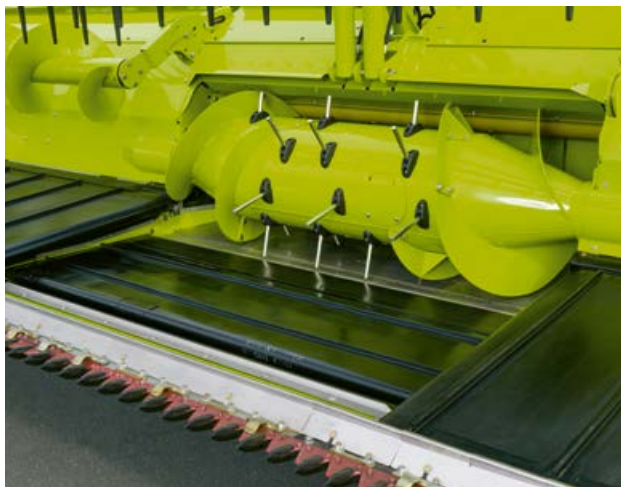
There is continuous automatic adjustment of the speed of the belts
