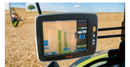
In the S10 terminal AUTO TURN can also create and work blocks automatically.
