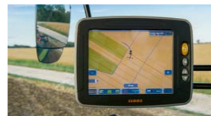
Standard on all GPS PILOT S10 and S7 terminals: TURN IN indicates to the driver the best track to take next based on speed and steering lock. When the driver activates the steering system, the machine follows the suggested path.
