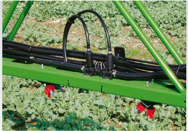
DUS pressure recirculation system
