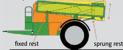
Sprung damping of the boom during transport
