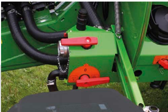
The venturi fast fill on the UX Special allows filling speeds of up to 500 l/min.
