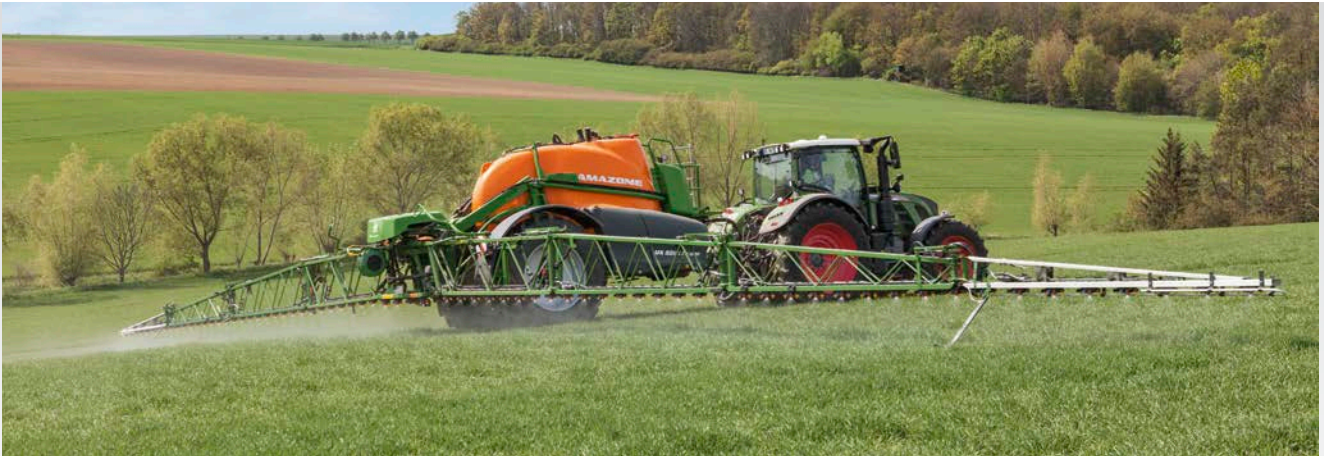
ContourControl with negative boom angling
