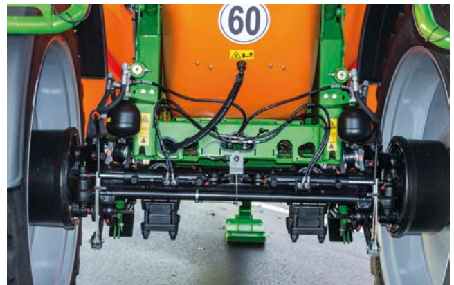
Hydro-pneumatic axle suspension with AutoTrail axle steering
