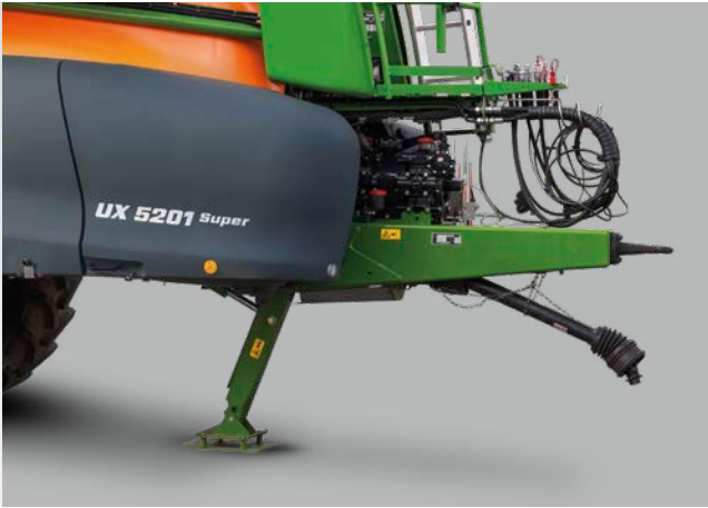
Top mounted drawbar with towing eye and hydraulic parking jack
