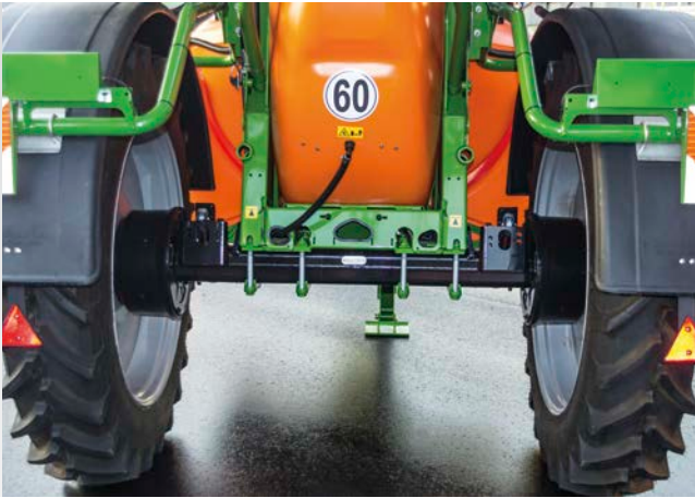
Rigid axle with track widths of 1.50 m to 2.25 m
