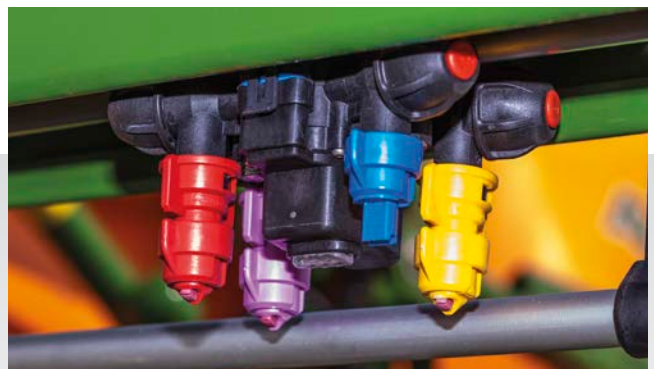
✔ AmaSelect electric individual nozzle control
