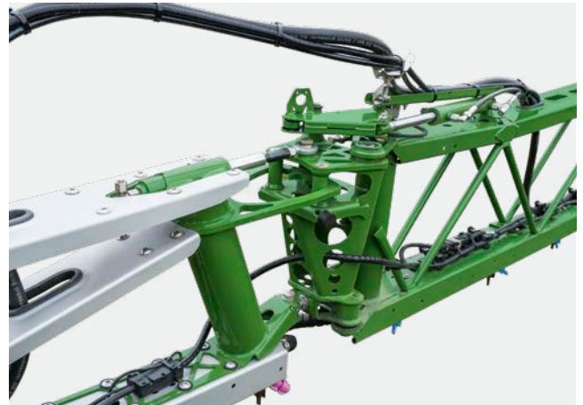
Hydraulically pre-tensioned break back joint at the boom end which works on a saloon door principle
