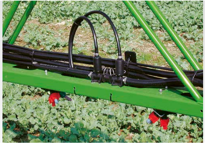
DUS pressure recirculation system
