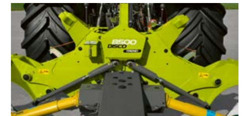
Compact, robust mounting block with integrated ACTIVE FLOAT suspension system as standard.
