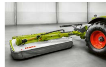
With hydraulically controlled booms, working widths of between 9.40 and 10.70 metres can be achieved, according to the front mower used.
