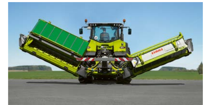
Professional control system provides individual lift and folding capability.
