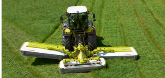
Individual lifting function for mowers at the headland.
