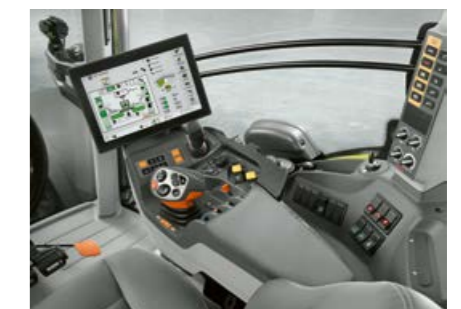
If the tractor is equipped with an ISOBUS-capable terminal, preselection control for the CONTOUR can be handled straight from there.
