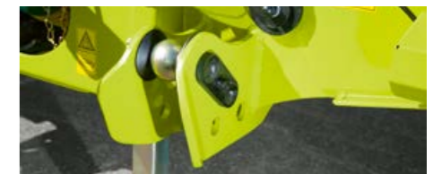
Lower link guide clips for ease of mounting.
