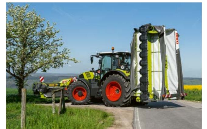
Less than 4.0 m high, and a compact package all round, like all DISCO models. The two mowers retract telescopically, and the machine then folds into the road transport position.
