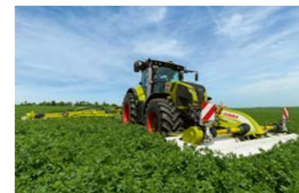
Additional options for the front mower, e.g. speed monitoring, ACTIVE FLOAT control and protective cover folding.
