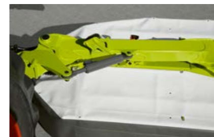
Hydraulic non-stop breakback protection in case of a collision impact – the mower pivots, and is automatically placed in the starting position.
