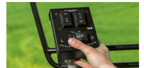
The DISCO 1100 TREND also has a practical control unit for the individual lift function, for folding into the transport position, and, as an option, for switching the work lights on and off.
