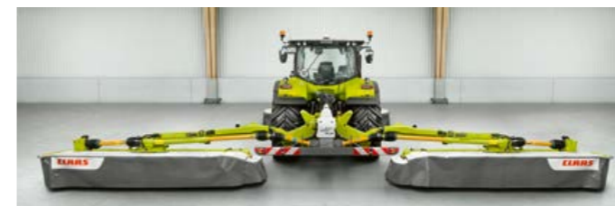
Two hydraulically controllable telescopic booms with continuous adjustment for optimal overlapping in the DISCO 1100 TREND.
