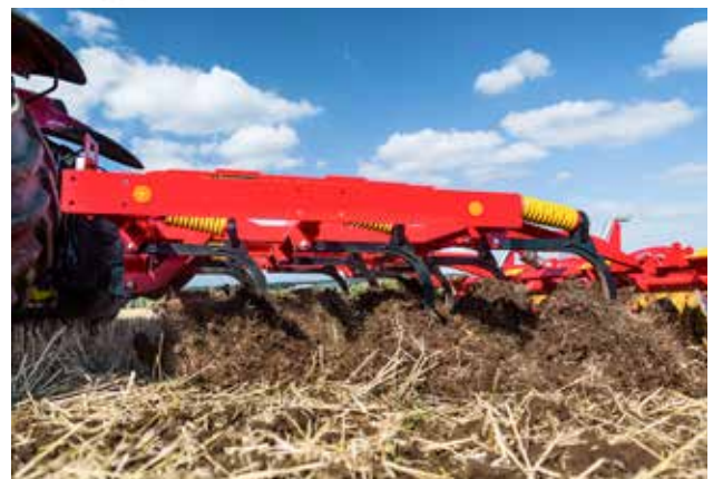
The Cultus tine is able to work with high performance down to 25cm working depth.
