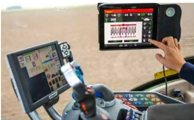
Seed is metered by two Fenix III units, each metering one half of the machine, this enables half machine shut-off from the cab.
