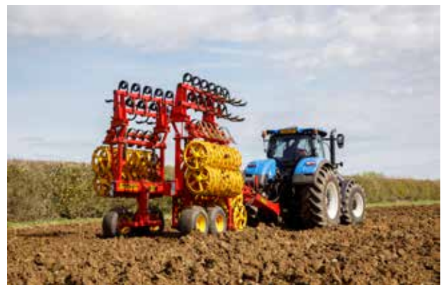
The Väderstad folding gives RexiusTwin low center of gravity and good manoeuvrability in transport, as well as excellent contour following in the field.
