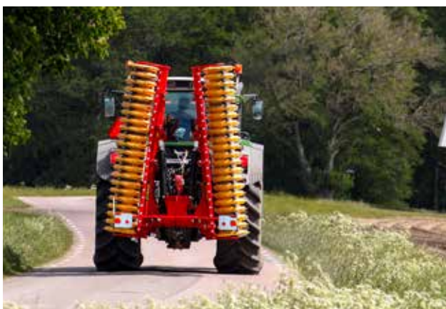
The transport width of Carrier X is only 2.4m and even when folded, you maintain a good rear view from the cab.
