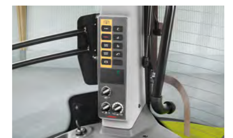
PTO speeds and the electronic linkage control system can be adjusted on the B-pillar.
