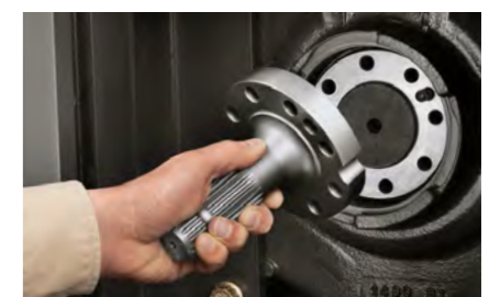
The PTO stub can be changed easily.
