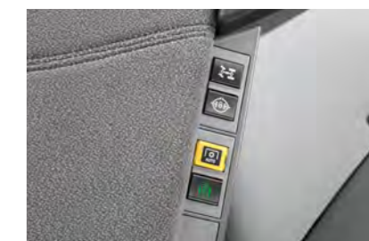
Switch to activate front axle suspension.
