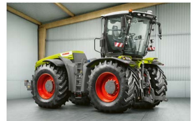
The TRAC VC has the most convenient reverse-drive system on the market. Its cab can be rotated through 180° in less than 30 seconds.
