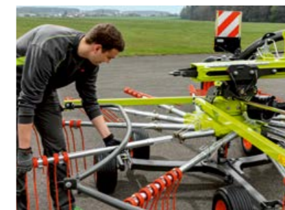
PROFIX tine arm attachment system.
