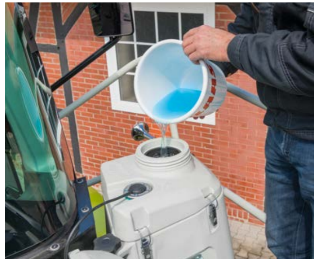
Filling the silage additive tank
