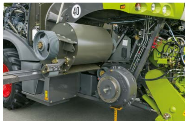
Easy removal and installation of the accelerator
