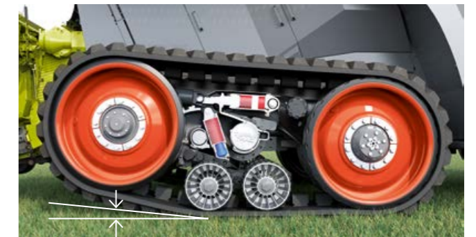
66% contact area: the track roller is raised by up to 100 mm.
