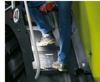
LED step lighting for safe access to the comfort cab
