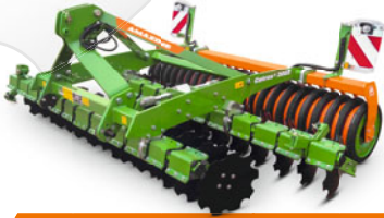
Catros rigid or folding mounted compact disc harrows
