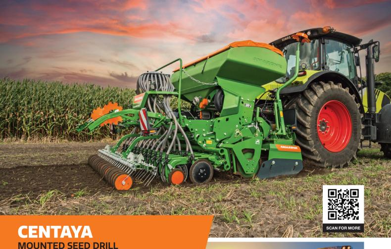
The Centaya pneumatic harrow-mounted seed drill is the ideal tool for precise sowing. In combination with the a rotary harrow or rotary cultivator, the seed drill, in working widths of 3m, 3.5m and 4m, creates an ideal seedbed.
