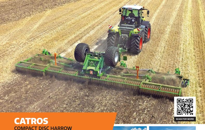
The Catros range of compact disc harrows are ideally suited for shallow and intensively mixed soil tillage. Thanks to its easy pulling and working widths from 3–12 m, especially high forward speeds, impressive work rates are possible.
