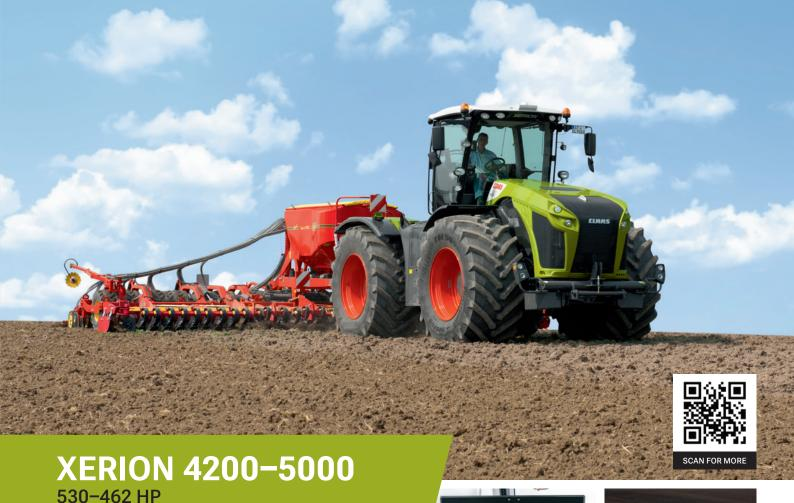
Uniquely designed for maximum slip control, tractive performance, and dynamism. A Mercedes-Benz engine efficiently delivers up to 530hp from a CMATIC continuously variable transmission, with four equal-sized wheels or dual tyres that convert engine power into tractive power. Intelligent systems combined with intuitive operation via the CEBIS touchscreen display, well-appointed suspended cab with excellent visibility, and long service intervals,
