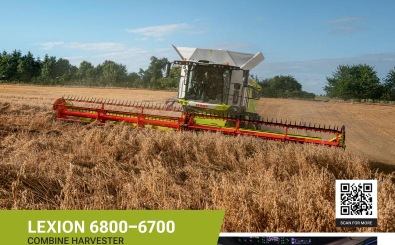
Featuring an accelerated crop flow enabled by APS and an additional separator drum after the threshing drum, the LEXION 6000 represents a new category in the straw-walker machine segment. Benefit from stable harvesting performance along with excellent straw quality.
