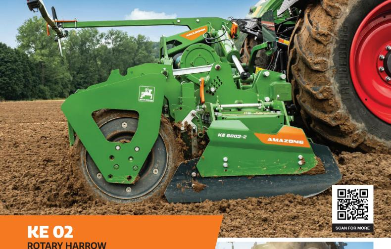
Robust and light at the same time, KE 02 Super is the right machine for the demanding requirements of a modern arable farm. A strong frame, one-piece rotor head and shaft, and a sprung tine fixing, make the KE 02 rotary harrow superbly suited for soil tillage after plough and mulch sowing on precultivated soils.
