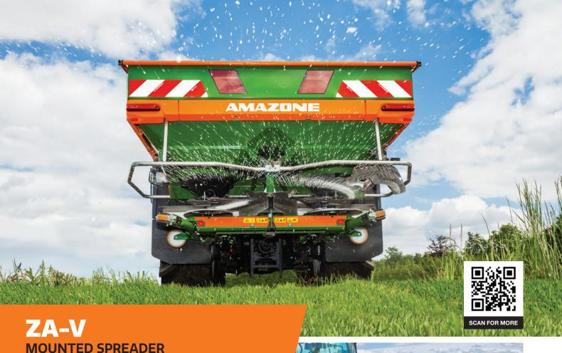
A state-of-the-art fertiliser spreader with hopper capacity from 1,400 to 3,200L, reaches high working speeds of up to 30km/h. Thanks to its high application rate of up to 390kg/min and a working width of up to 36m, it achieves exceptionally high work rates.
