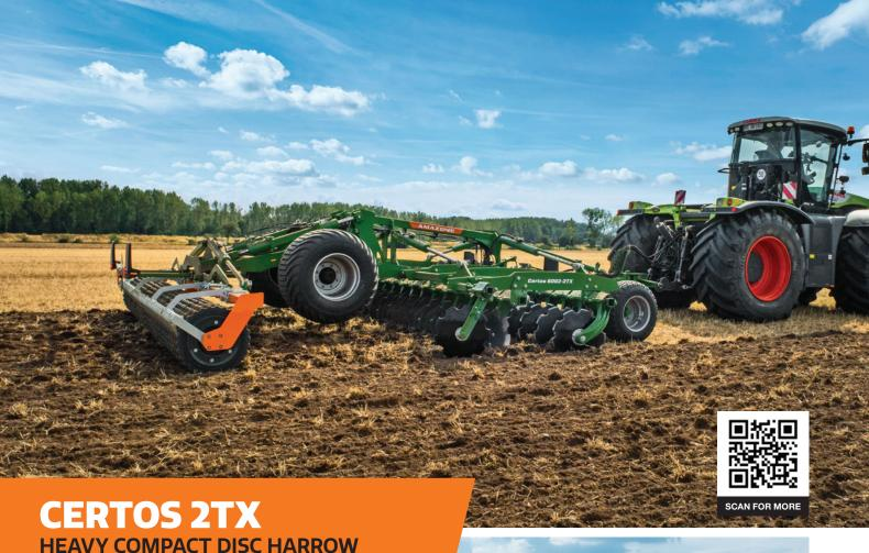
The Certos-2TX is ideally suited for intensive mixing and medium to deep soil tillage. With its 660mm discs, the Certos-2TX penetrates the soil down to 20cm and incorporates large amounts of organic matter, blockage-free. A powerful allrounder for any farm thanks to its wide application range, and working widths of 5–7m.
